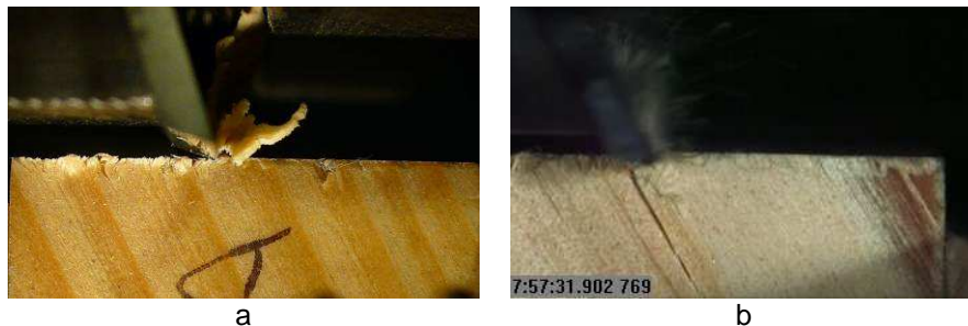
Figure 10. Douglas Fir processed at -60° of grain angle at low (a) and high (b) speed, with 0,2 mm d.o.c.
