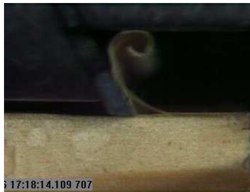
Figure 5. Dougls Fir processed at high speed with 0,2 mm of d.o.c.
