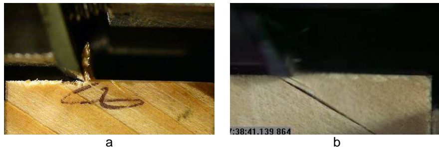
Figure 8. Douglas Fir processed at -30^\circ of grain angle with low (a) and high (b) speed with 0,2 mm d.o.c.
