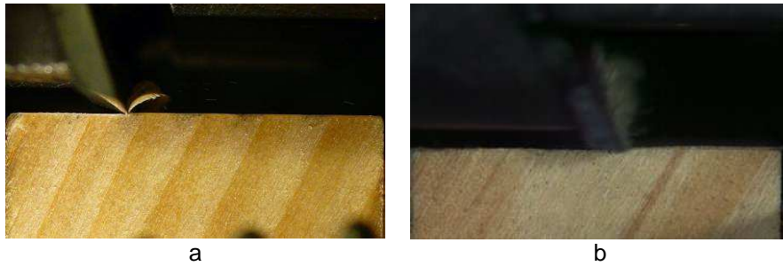
Figure 9. Douglas Fir processed at 60° of grain angle at low (a) and high (b) speed, 0,2 with 0,2 mm d.o.c.
