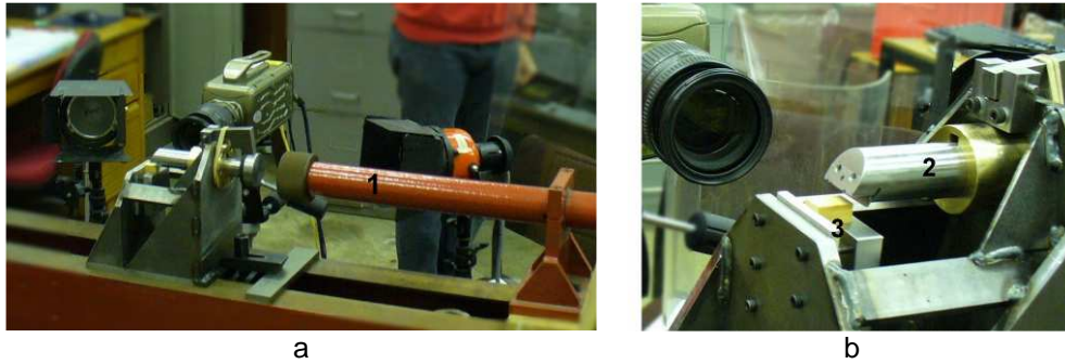
Figure 2. The adapted Hopkinson's Bars system used in the high speed tests.
