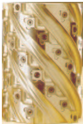
Figure 1 - Carbide tipped knives on the special helicoidal cutter head
